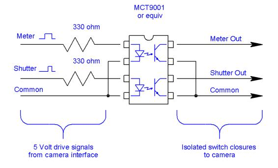
The optiosolator in this circuit is a common Fairchild MCT9001 (available from Mouser or Digikey with that part number). Any 2 channel optoisolator will do, so long as it is a "passive" open collector type, and not an active "logic output type" (open collector types mimic switch closures as outputs, while logic types provide an active logic signal as outputs)
