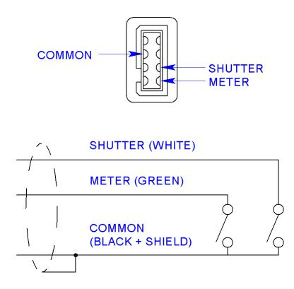
Notes: Cannibalize genuine Nikon MC-DC2 remote switch. This connector has very tiny, precise, parts, and the aftermarket switches we've seen are nowhere as precisely made as the original Nikon switches, and tend to have a loose fit with unreliable retention.
