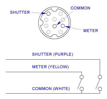
Note: because this is a threaded locking connector, aftermarket switches seem to be equally reliable in this application, but note – if you're using an aftermarket switch, wiring colors may vary, so double-check your wiring.
