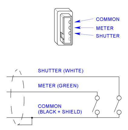
Notes: Cannibalize genuine Nikon MC-DC1 remote switch. This connector has very tiny, precise, parts, and the aftermarket switches we've seen are nowhere as precisely made as the original Nikon switches, and tend to have a loose fit with unreliable retention.
