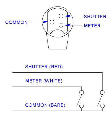
Notes: Cannibalize genuine RS-80N3 Canon remote switch. The real Canon part uses an delicate but reliable expanding ring-sleeve for very positive locking, whereas aftermarket switches seem to depend on a friction fit and tend to work loose.
