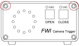
Then remove the top 2 case screws on the front panel, and all 4 case screws on the rear panel.
