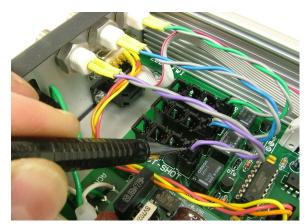
The logic level, active hi, 5 volt outputs are the connector row that is closest to the rear of the unit.
